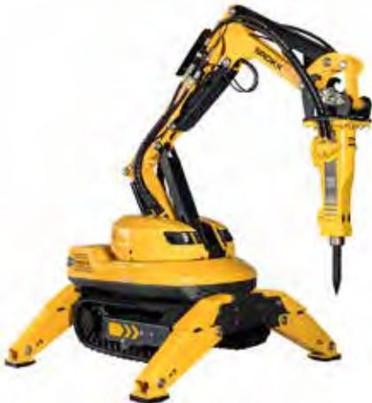
The new Brokk 110 demolition machine delivers 15 percent more power than its predecessor, the Brokk 100, without sacrificing the compact size and versatility for which the company's machines are known.
