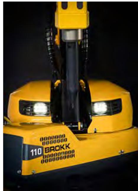
The Brokk 110 features hardened parts, LED headlight protection, reinforced corners and a new steel gray color coating in strategic areas to add additional resistance to dirt and scratches.
