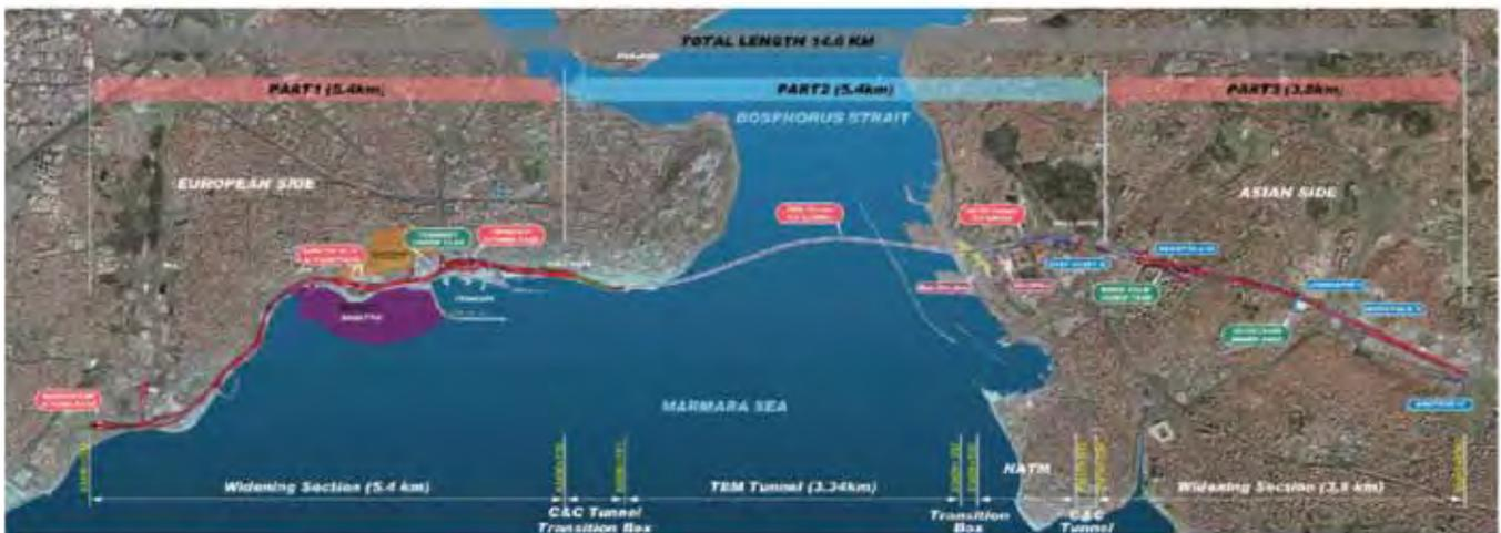
The 13.2 m (43 ft) external diameter, double deck Istanbul Strait Road Tube Crossing is one of the most challenging underwater tunnel projects in the world. Subjected to 11 bars of hydrostatic pressure, variable geology, and being in a very active seismic area, the execution of the project required innovative solutions, sophisticated construction techniques and
