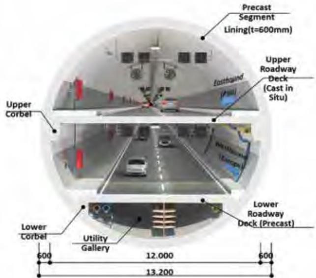
with precast concrete panels resting on similar corbels. The space beneath the lower deck accommodated the cableways, sump pumps, water and drainage systems, and other utilities supporting the tunnel operation.
