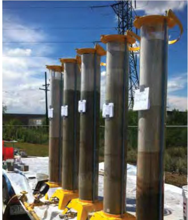
water: cement ratios. The first batch consisted of OPC at a water cement ratio of 1:1. For the next batches, ultrafine cements were used and the water content was increased by 0.5 each time for the next three ultrafine mixes. Inspection of each new batch of grout mix was conducted and results recorded. The information recorded included quantities of cement
